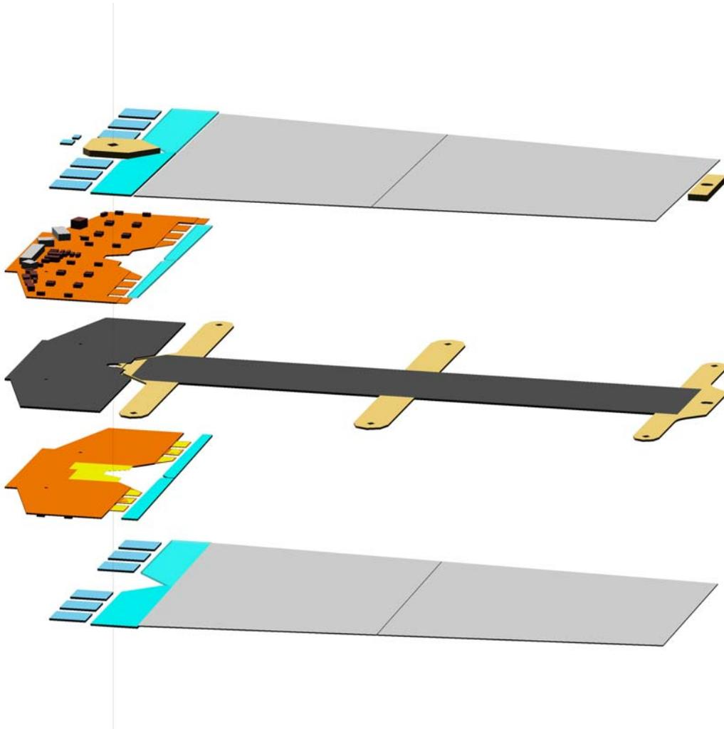
*Figure 1: Exploded view of module components with spine as central mechanical structure, sandwiched between the silicon detectors.*
