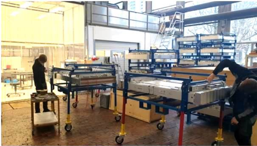
Figure 36: sMDT chambers in various stages of completion in the construction hall in the old MPP building in Munich. After the assembly out of the drift tubes, the gas connections to each individual drift tubes are installed. More than 5000 rubber sealing rings each chamber have to fullfill very high gas tightness standards. By design this worked almost every time in the first attempt. Afterwards, the readout electronics boards and Faraday cages protecting them are installed. The teststand for the final certification test with cosmic ray muons in visible in the background of the pictures.
