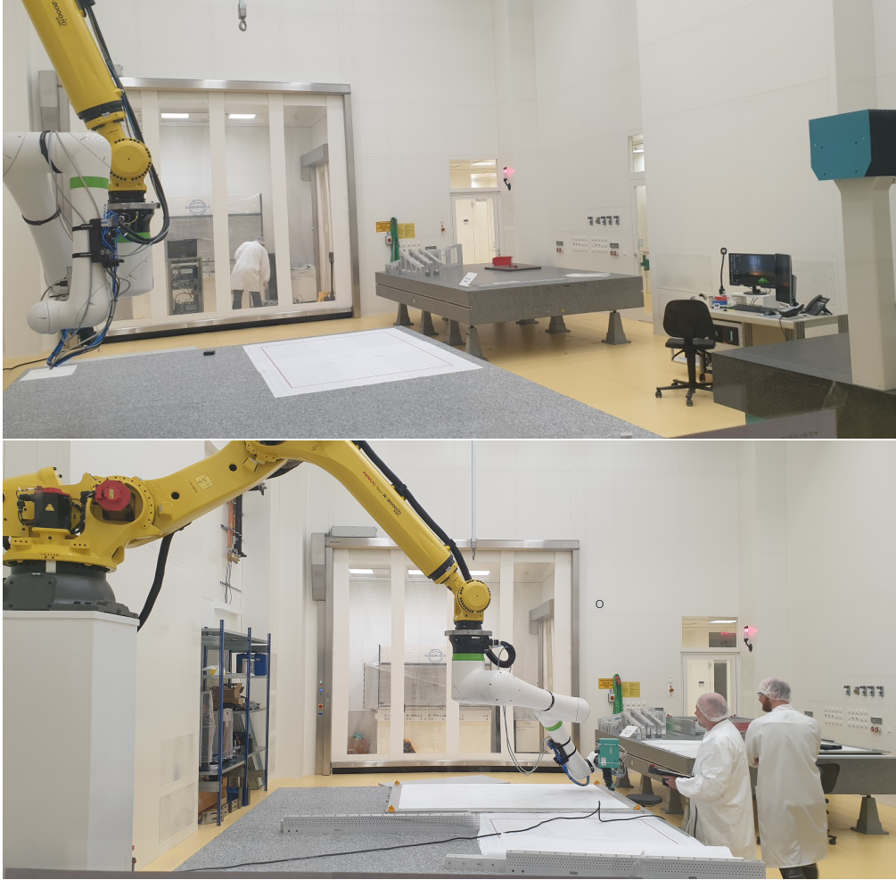
Figure 42: Top: Detector construction facility in a temperature controlled clean room at the new MPP building on the MPG campus in Garching in operation since the beginning of 2024. Large sMDT and RPC detectors will be constructed on polished granite tables using high-precision mechanical jigs and automatized robotic devices. The automated coordinate measuring machine is visible on the right. Bottom: The glueing robot in action on the assembly table for sMDT and RPC detectors.
