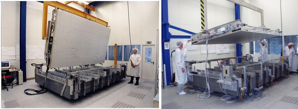
Figure 27: Left: The first MDT prototype chamber constructed at MPP in the new clean room in February 1998. The chamber dimensions are of the same size as for the series production. Right: Assembly of the first MDT chamber of the series production at MPP with the first prototype chamber in August 2000. The drift tubes of each layer are positioned in precise combs on the granite table. In the picture, the first tube layer has been glued to the support frame which has been lifted from the table. The support frame with glued tube layers can be rotated on the crane in order to successively glue the next tube layers to the top and bottom of the frame. The construction of the 88 chambers required for the outermost barrel layer of the ATLAS muon spectrometer was completed in December 2005.
