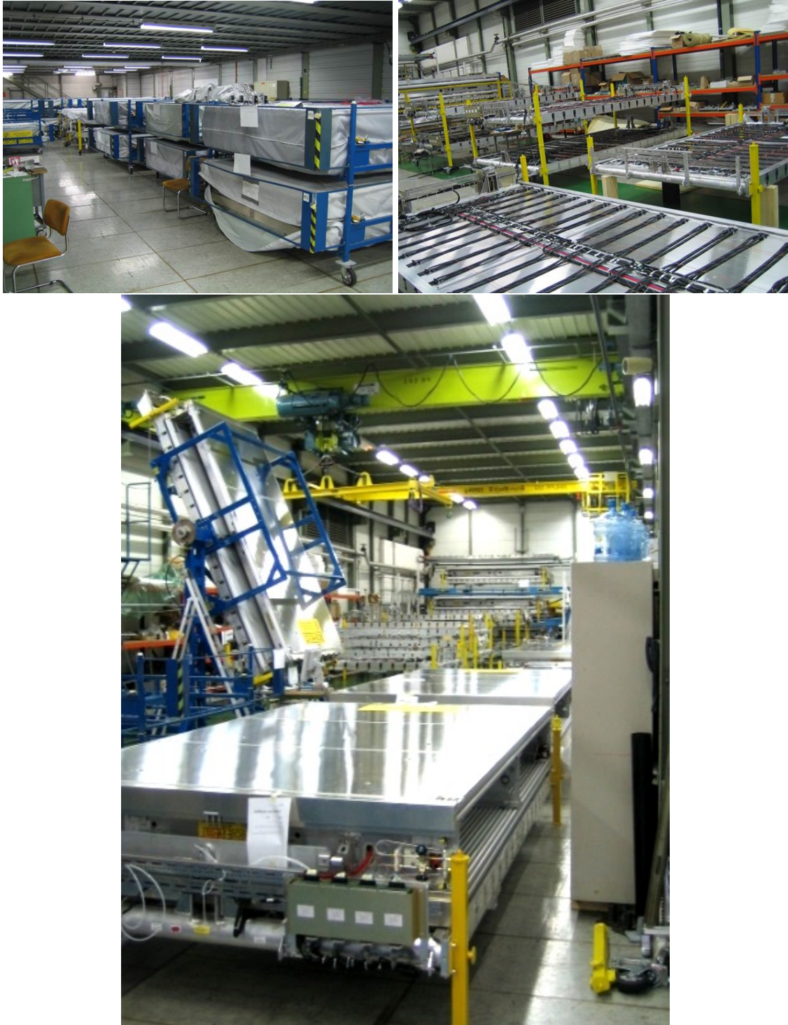
Figure 30: Integration of the MPP MDT chambers with RPC trigger chambers and commissioning in a dedicated hall at CERN before installation in the ATLAS detector. Top left: MDT chamber storage at CERN. Top right: RPC chambers prepared for the integration with the MDT chambers in support frames designed and constructed at MPP. The distance between MDT and RPC chambers in the package had to be adjusted with millimeter precision under the same inclination angle as in the muon spectrometer to make the installation in the small available space possible. The rotation stand used for this purpose is visible at the top left in the picture at the bottom. The row of completed combined detectors can be seen in the foreground.
