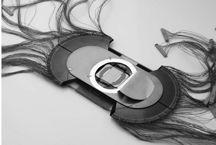
Figure 2: Photo of the first silicon strip detector made in planar technology. This detector was used in the NA11/NA32 experiment. The sensor's sensitive area is 24 \times 36 \text{ mm}^2 . The sensor is embedded in a large fan out board providing cable connections to individual amplifiers.
