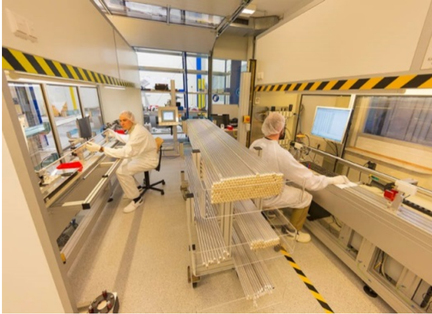
Figure 34: Clean room at MPP for the semi-automated assembly of the drift tubes of the sMDT chambers. The wires are fed through the tubes using air flow to avoid any manual contact and are tensioned with high reproducibility to guarantee equal gravitational sag of the wires in all tubes within 4%.
