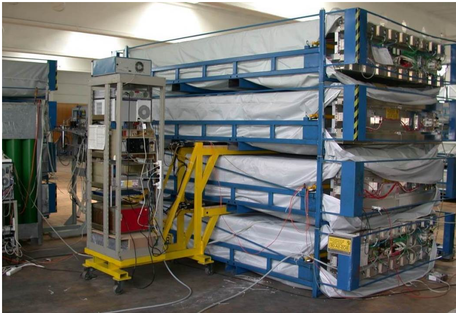
Figure 28: MDT chamber storage and test with cosmic ray muons during the series production in a large hall rented in the north of Munich while storage space for the chambers was not yet available at CERN.
