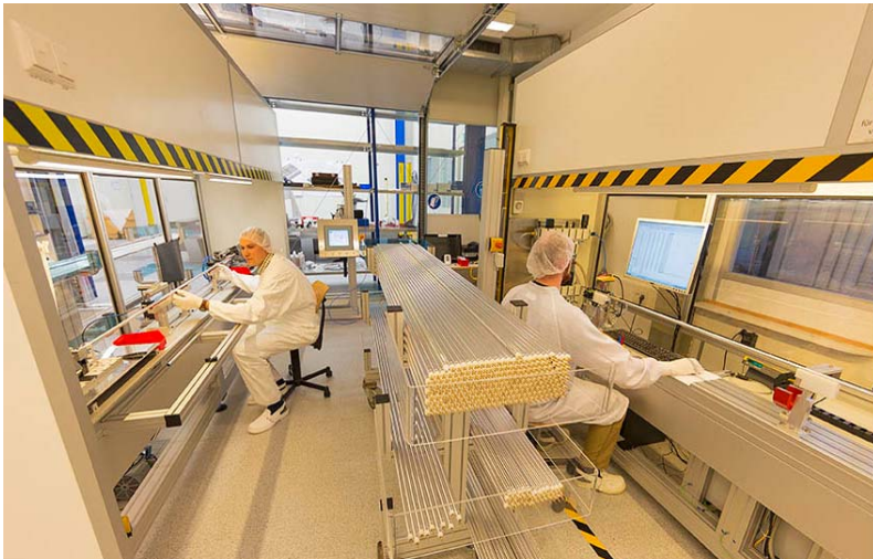
New drift tube assembly facility at MPP
