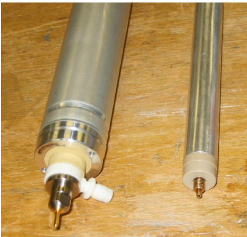
15 mm \varnothing sMDT tubes instead of 30 mm \varnothing MDTs
