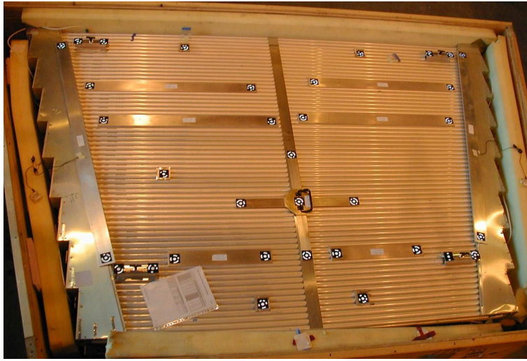
Fig. 12: Photo of an MDT chamber during the photogrammetry measurement. Five coded targets on a cross at the center define the (arbitrary) photogrammetry coordinate system; scale bars with two targets at their ends, positioned in various places, constrain the length scale. Adapters for two targets each are mounted on the sensor platforms near the four corners of the chamber (this type of chamber, EML2, has four rail mounts), and the four single targets on small plates near the long and short sides are the survey targets. The magnetic-field sensor platforms are missing.
