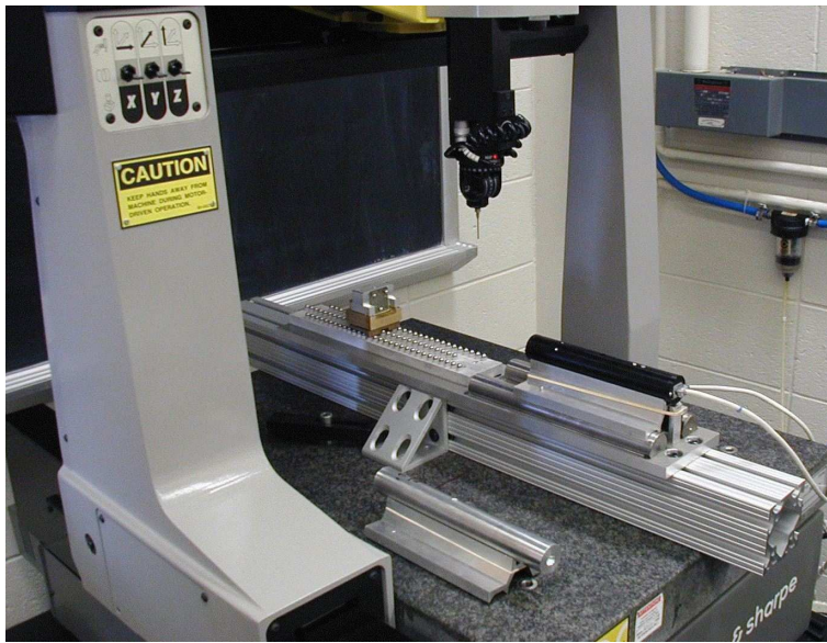
Fig. 9: The calibration stand for the proximity sensors while being measured with a CMM. This stand is used for calibrating both cameras and masks. It consists of a rail mount for the camera, and about 30 3-ball mounts at different distances from it for a brass interface plate on which the mask is mounted.
