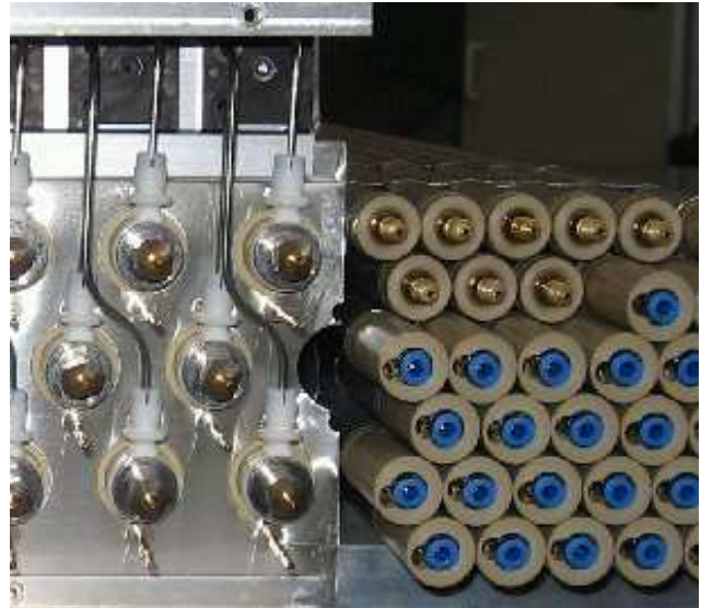
Figure 1.11: Front view of bundles of drift tubes with 30 mm (left) and 15 mm (right) diameter.
