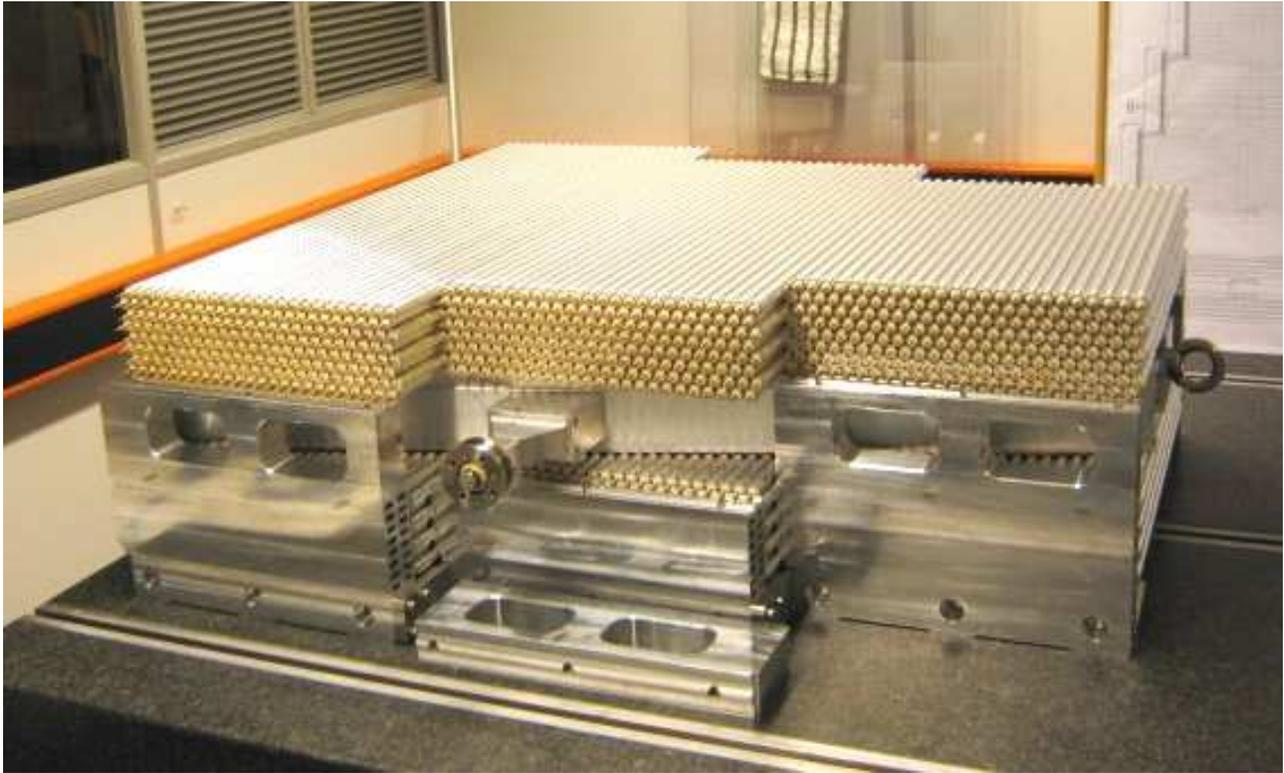
Figure 1.83: The small tube prototype chamber after assembly, consisting of two packages of 8 tube layers, with 72 tubes per layer and 1152 tubes in total.
