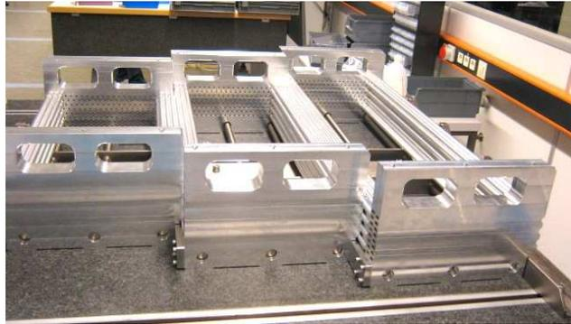
Figure 1.82: Precision placement of the small MDT tubes in high accuracy 'combs' before gluing with epoxy.
