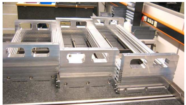
Figure 6.67: Precision placement of the small MDT tubes in high accuracy 'combs' before gluing with epoxy.
