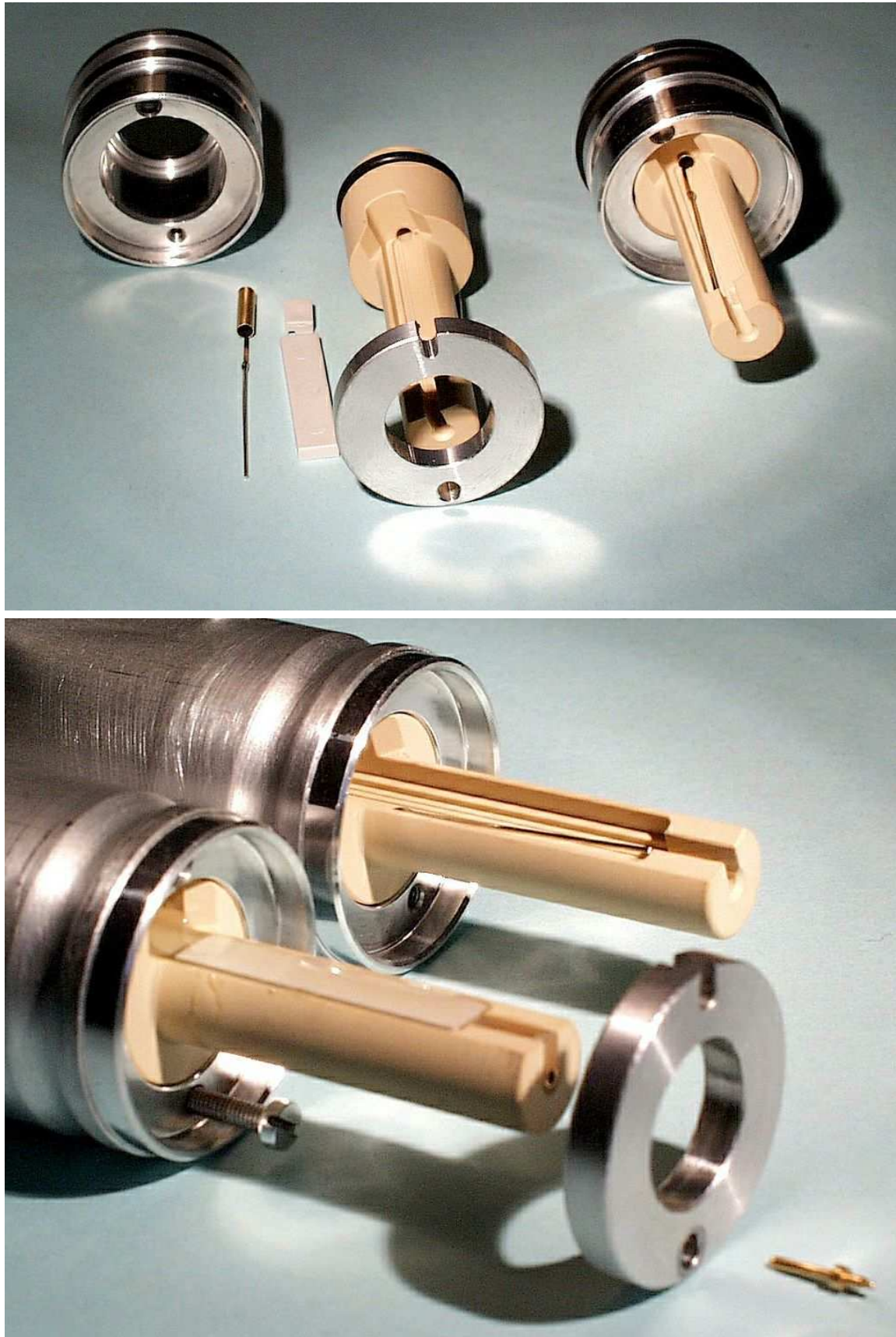
Figure 3: Endplug and drift tubes for the BOS prototype chamber.
