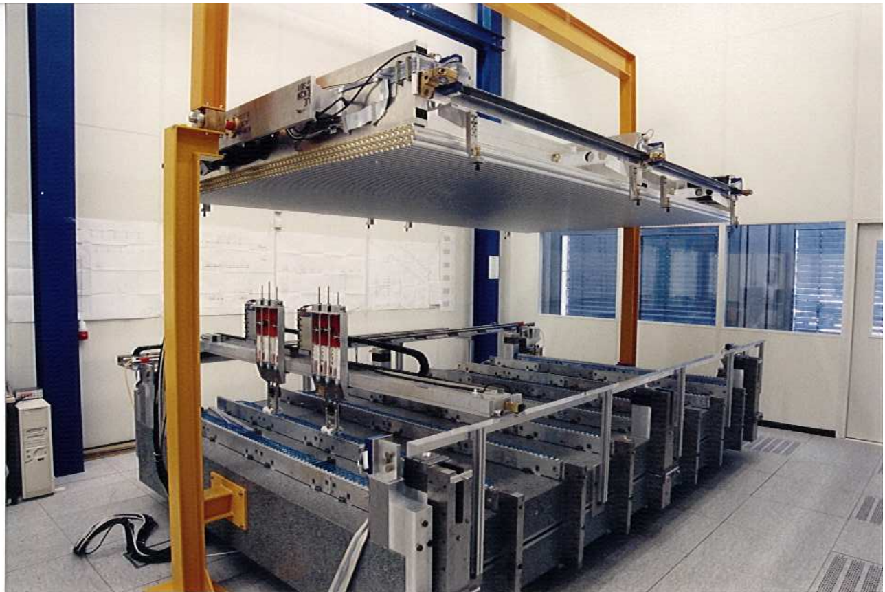
Figure 28: The BOS prototype chamber during assembly with the first multilayer completed. The glue dispenser with its two moveable heads is installed for the next tube layer.
