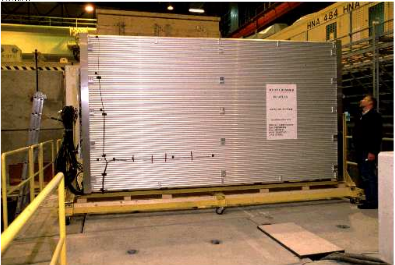
Figure 30: The BOS prototype chamber after completion set up in the test beam area at CERN.
