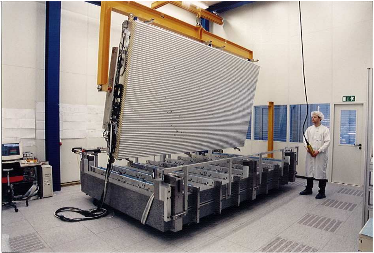
Figure 29: Rotation of the BOS chamber on the crane during assembly.
