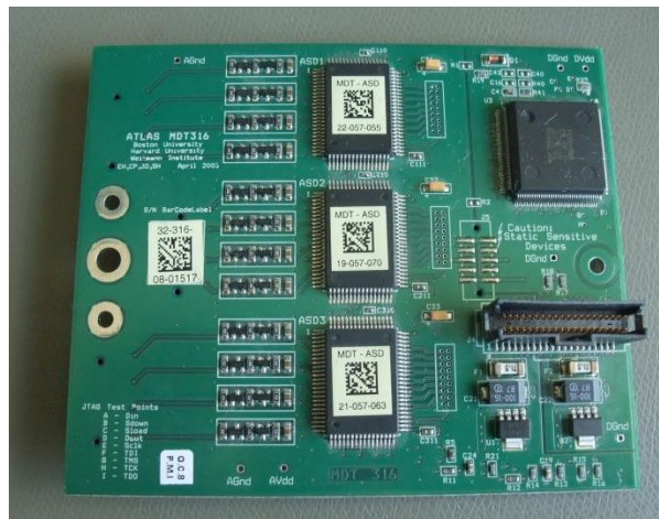
“Old” mezzanine card (MDT316) with AMT and no FPGA.
