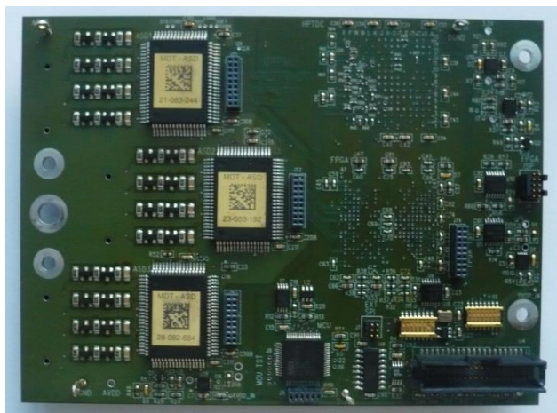
“New” mezzanine card (MDT_FPGA_R2) with HPTDC and FPGA. It can generate trigger data.
