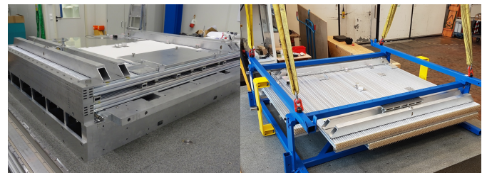
Figure 5: BIS 78 sMDT chamber (left: completed on the assembly table, right: in the transport frame).
