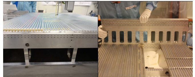
Figure 4: sMDT assembly jigs (left: BIS 78, right: BMG) with precise hole matrix for positioning of the endplug reference surfaces and, therefore, of the sense wires. A multilayer of drift tubes can be completed within one working day. The multilayer distance is also precisely determined by the jig.
