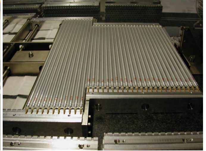
(b) Lay-up of the first tube layer.
