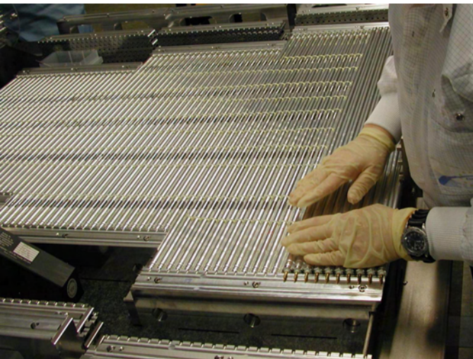
(c) Gluing of the second tube layer onto the first one.
