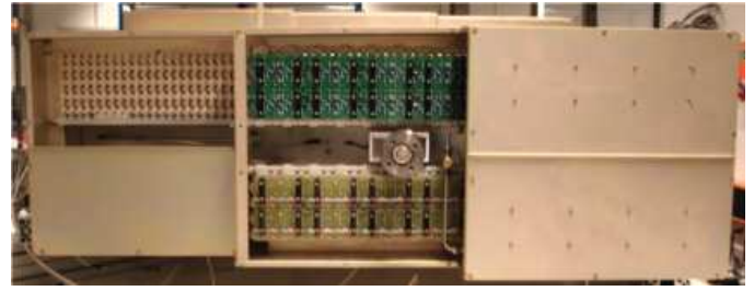
Fig. 5. Photograph of the prototype chamber showing the open Faraday cage, the gas system, and the HV and readout adapter cards.
