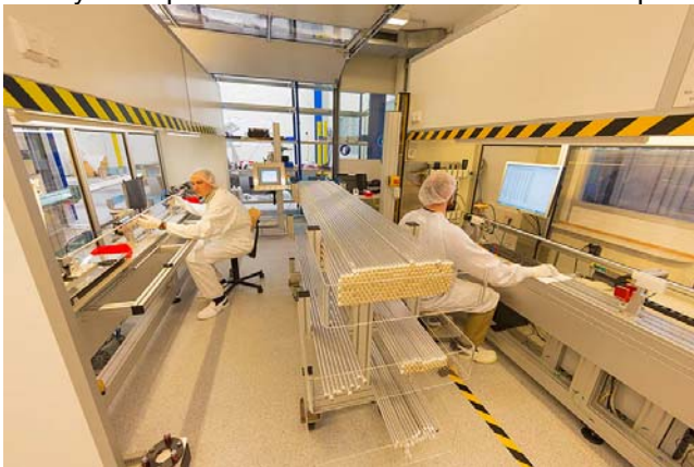
Figure 3: Top left: Semi-automatized drift tube assembly in a climatized clean room. On the same room the drift-tube tests are performed (see text).
