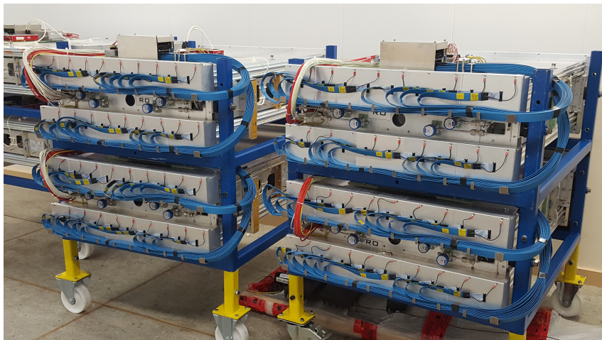
Figure 24: Readout side of SMDT chambers (BMG chambers during commissioning at CERN) with closed Faraday cages and flat (blue) twisted-pair signal cables connecting the mezzanine cards to the externally mounted readout boxes (CSMs).
