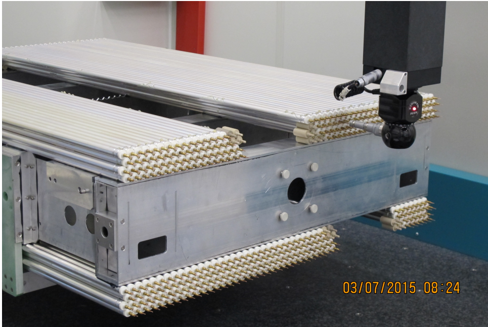
Figure 17: Measurement of the sense wire and alignment platform positions of a sMDT chamber with a Coordinate Measuring Machine (CMM). Individual wire positions are measured with an accuracy of 2 \mu\text{m} . The geometry parameters of the sense wire grids at the tube ends can be fully reconstructed. The wire positions on the readout and high-voltage distribution ends of the chamber are measured in the same coordinate frame allowing for the reconstruction of global deformations like torsion between the two ends.
