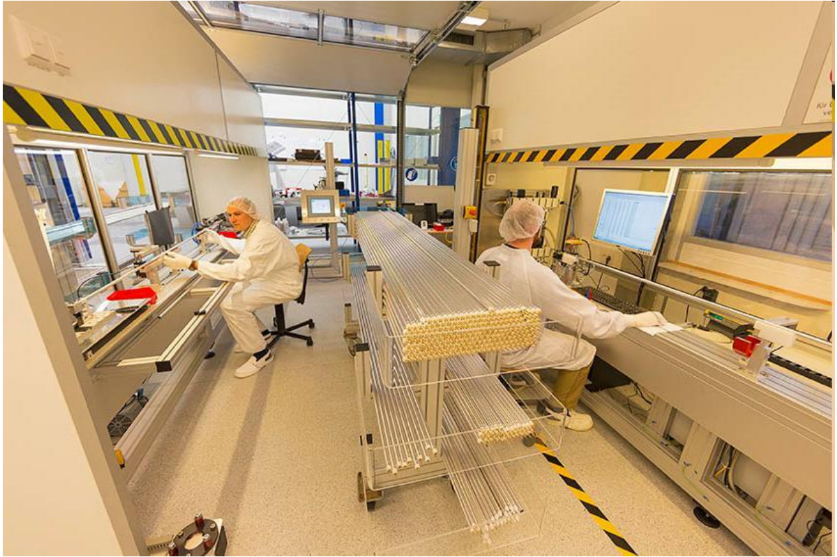
Figure 6: Semi-automated drift-tube assembly station in a climatized clean room.
