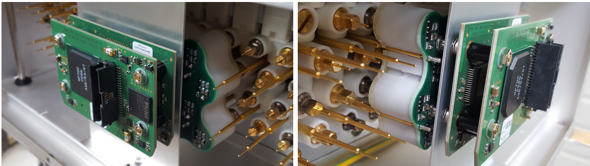
Figure 15: Left: sMDT signal distribution board with stacked mezzanine card carrying three ASD chips (middle layer) and the HPTDC with programming FPGA (top layer). The coupling capacitors to the signal pins of the drift tubes are encapsulated in injection molded white plastic containers to ensure high-voltage stability. The gold-plated signal pins and ground pins are inserted into receptacles on the signal distribution boards which also contain the protection network for the ASD chips. The passive signal distribution (hedgehog) board with the plastic containers is shielded from the mezzanine cards by an aluminum plate which is electrically connected to the outer Faraday cage. Right: sMDT signal distribution board with stacked mezzanine card mounted on the signal and ground pins of the drift tubes of a BMG chamber.
