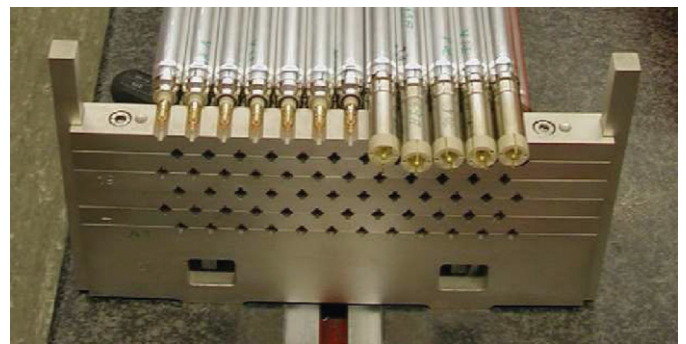
Fig. 5. Assembly of a prototype chamber with 15 mm diameter drift tubes. The external endplug reference surfaces at both tube ends are inserted in precise mechanical jigs (before the installation of gas connections and signal caps) in order to position the sense wires with better than 20\mu\text{m} accuracy.
