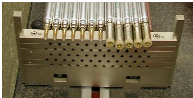
Figure 5: Assembly of a prototype chamber with 15 mm diameter drift tubes. The external endplug reference surfaces at both tube ends are inserted in precise mechanical jigs (before the installation of gas connections and signal caps) in order to position the sense wires with better than 20 \mu\text{m} accuracy.
