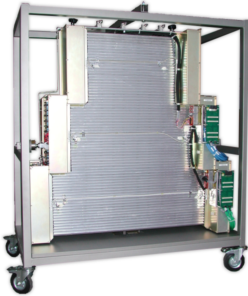
Figure 2: The sMDT prototype chamber of a size of one square meter.
