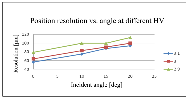
Figure 19: Resolution vs. incident angle as measured with muons in H8.
