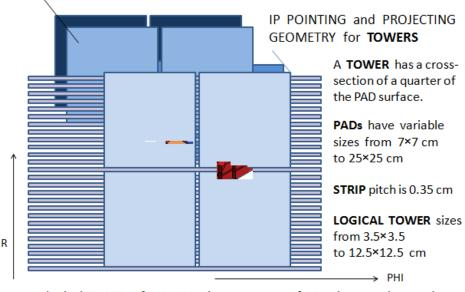
A logical TOWER of 4 PADS points to a group of 16 strips on a plane and  $4\times16$  strips in a logical tower.
