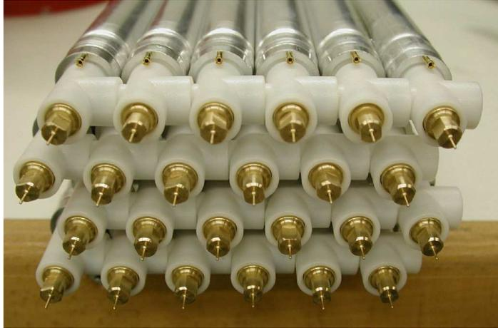
Figure 30: Picture of the gas manifold mounted on the prototype chamber.
