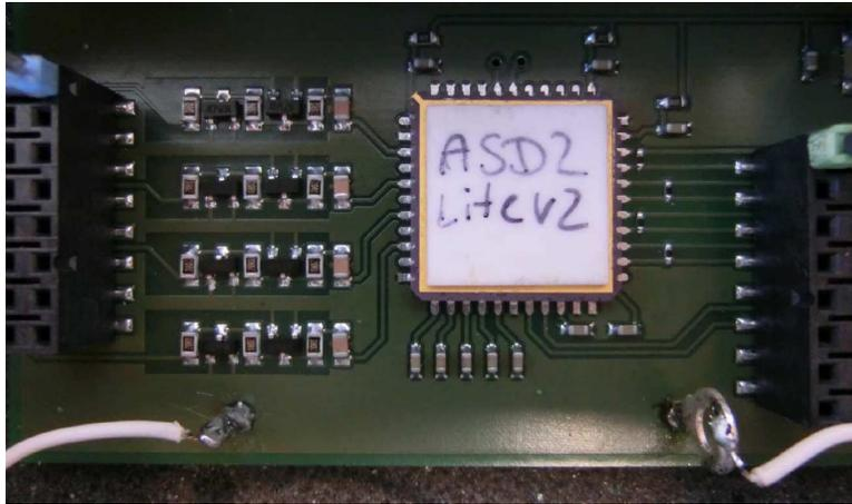
Figure 24: The new 4-channel ASD chip with full analog and digital functionality on the test board.
