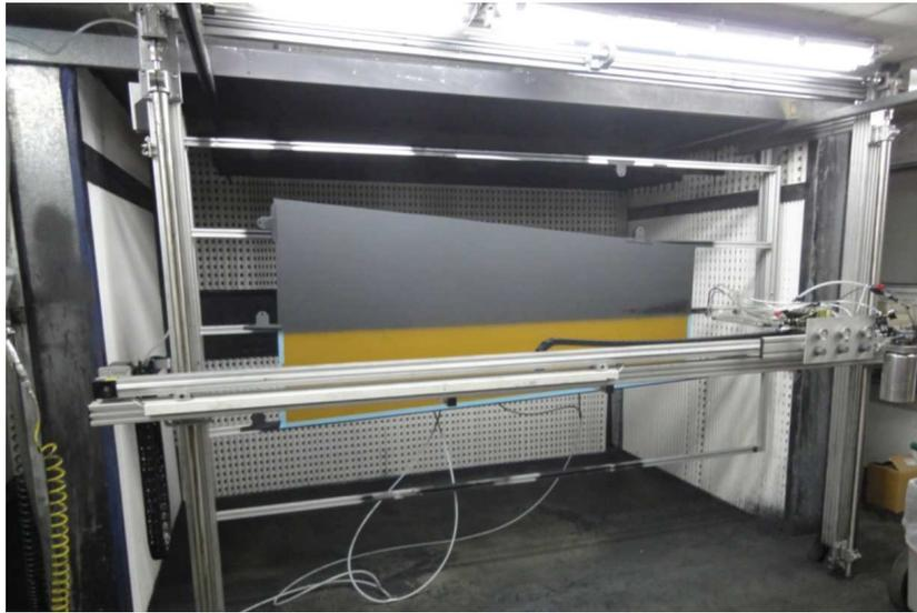
Figure 45: New fully automatic graphite spraying machine recently installed at the Weizmann TGC facility, in a fully controlled Temperature and Humidity room.
