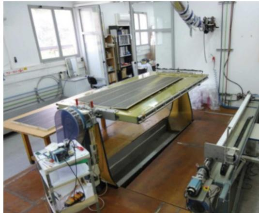
Figure 46: Left: new clean room to close TGC detectors. Right: improved wiring machine at the Weizmann TGC facility.
