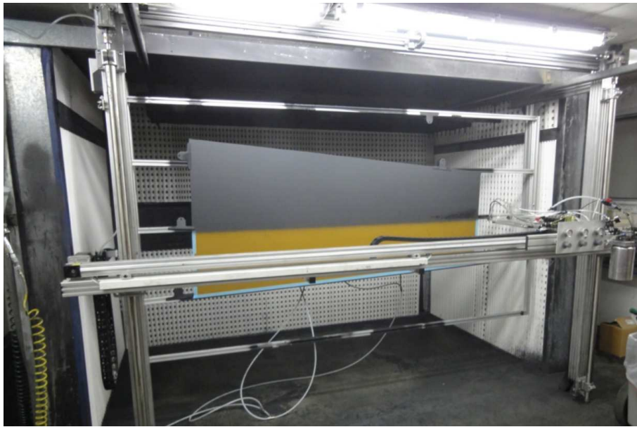
Figure 33: new fully automatic graphite spraying machine recently installed at the Weizmann TGC facility, in a fully controlled Temperature and Humidity room.
