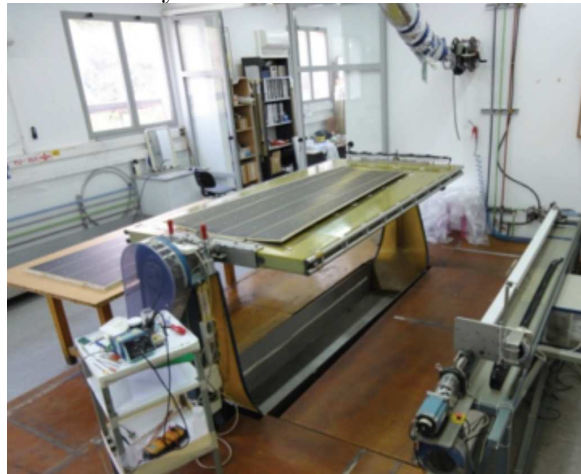
Figure 33: new fully automatic graphite spraying machine recently installed at the Weizmann TGC facility, in a fully controlled Temperature and Humidity room.
