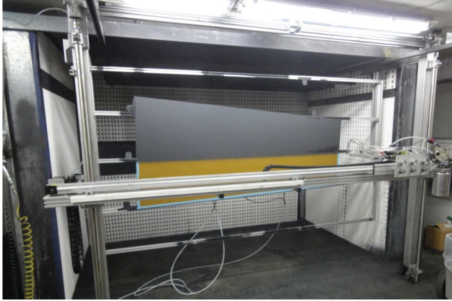
Figure 40: new fully automatic graphite spraying machine recently installed at the Weizmann TGC facility, in a fully controlled Temperature and Humidity room.
