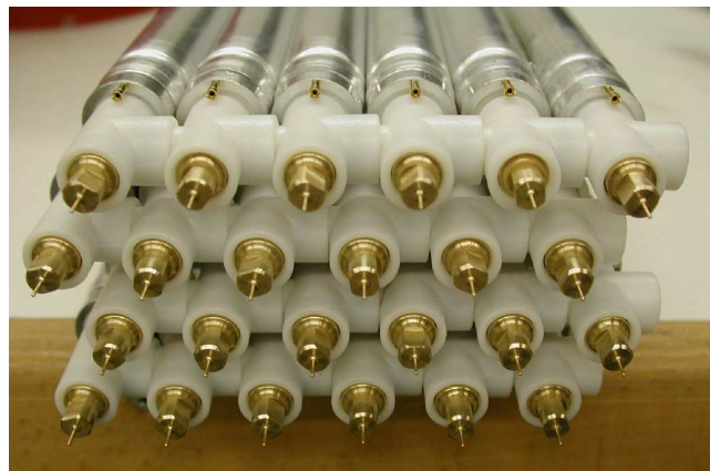
Figure 28: Picture of the gas manifold mounted on the prototype chamber.
