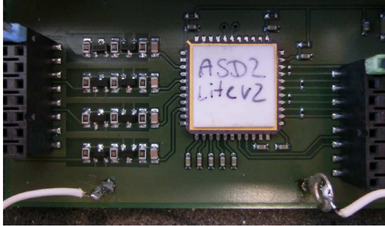
Figure 24: The new 4-channel ASD chip with full analog and digital functionality on the test board.
