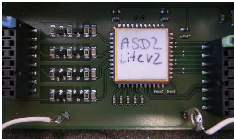
Figure 11: The new 4-channel ASD chip with full analog and digital functionality on the test board.
