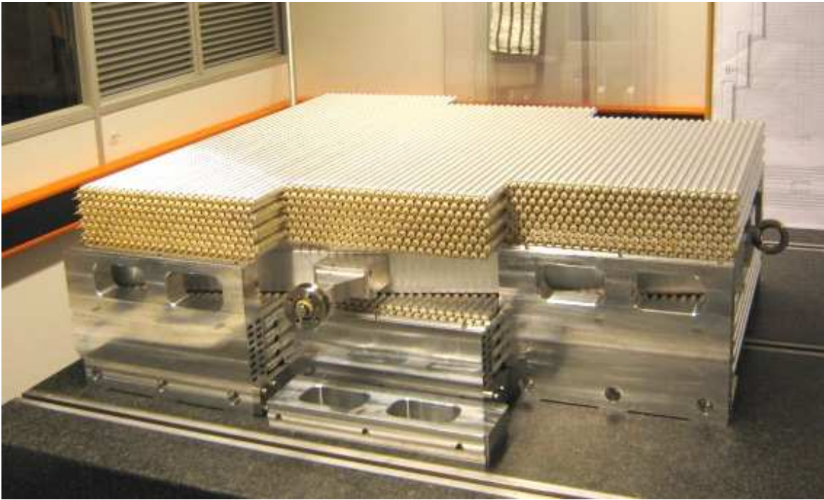
Figure 2: The small tube prototype chamber after assembly, consisting of two modules of 8 tube layers, 72 tubes per layer and 1152 tubes in total.
