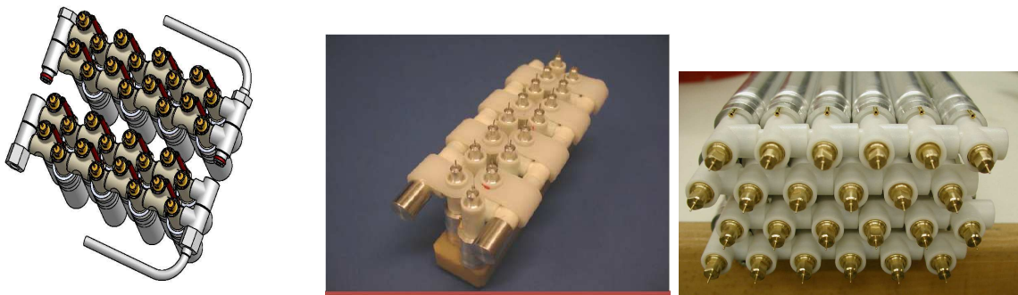
Figure 25: Two design models of the gas manifold (left) and a photo of the finished part (right)
