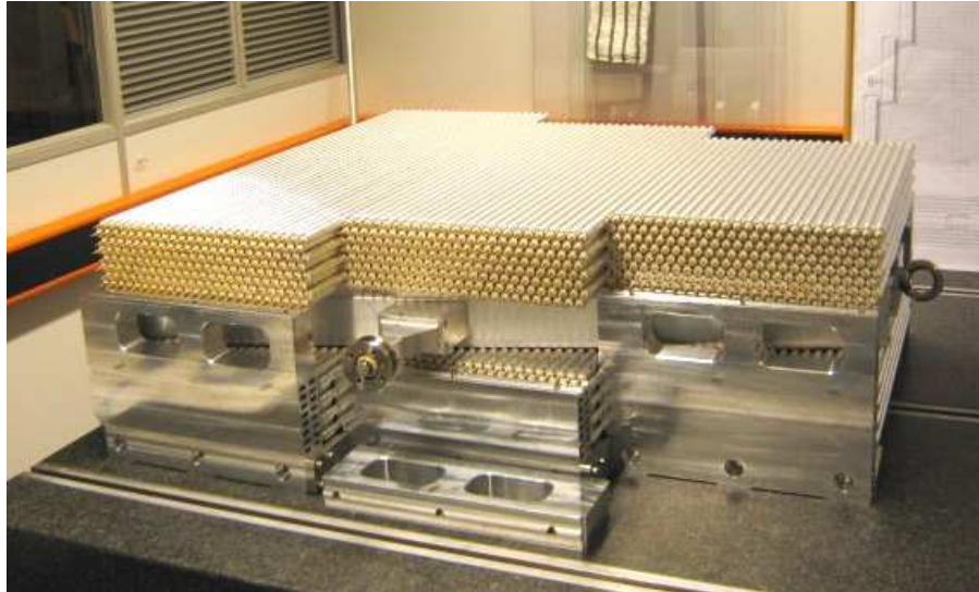
Figure 29: Assembly of the tubes into a sMDT chamber.
