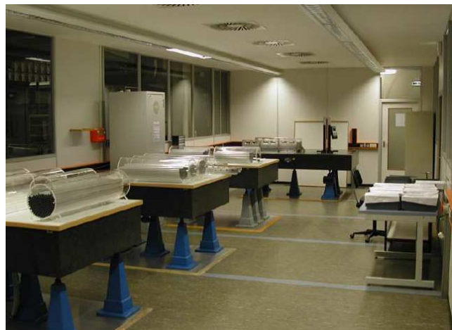
Figure 30: The small tube prototype chamber after assembly, consisting of two modules of 8 tube layers, 72 tubes per layer and 1152 tubes in total.
