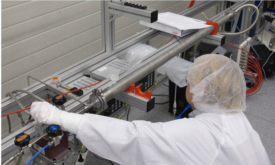
Figure 15: Gas leak testing. The central cylinder is the testing cylinder (“Torpedo”), which contains the tube. The lower left is the gas connection to the sMDT tube. The upper right leakage detector measures any gas which has leaked from the sMDT tube to the Torpedo.
