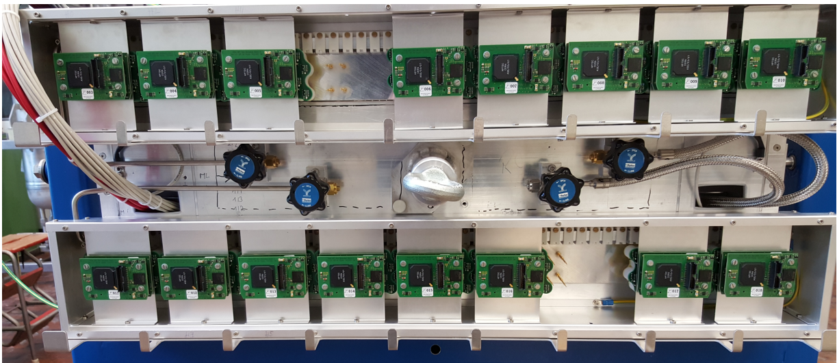
Figure 46: Chamber with readout system installed. Note: the two gaps correspond to the cutouts required for the ATLAS alignment system. In the center are the four valves, two for gas in (left side of the chamber) and two for gas out (right side of the chamber).
