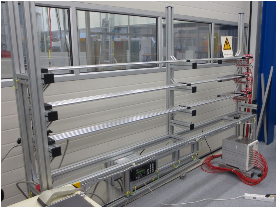
Figure 17: HV testing apparatus. This setup can test up to 15 tubes simultaneously. On the bottom right is the HV source connected to each chamber with individual current measurements for each tube.
