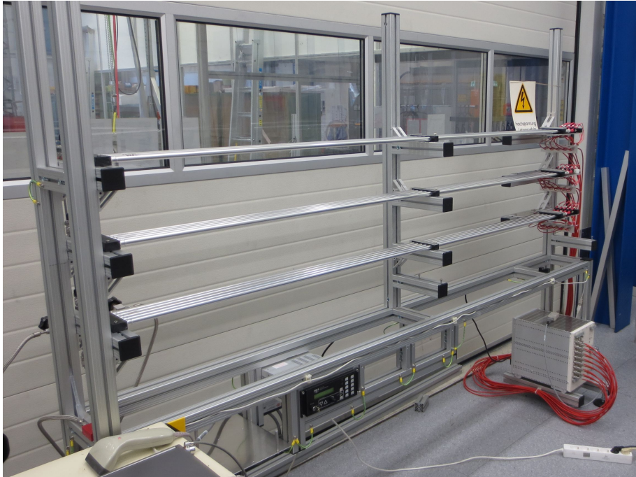
Figure 15: HV testing apparatus. This setup can test up to 15 tubes simultaneously. On the bottom right is the HV source connected to each chamber with individual current measurements for each tube. The right hand side is seen in Fig. 13. The pipes are also connected to a gas bottle to bring the tubes up to 3 bar pressure (absolute) for the testing of the dark current. A sample plot showing the voltage and current on five of the tubes can be seen in Fig. 16.
