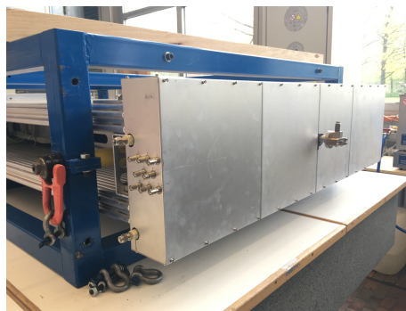
Figure 33: Completed chamber with Faraday cages seen from HV side (left) and RO side (right).
