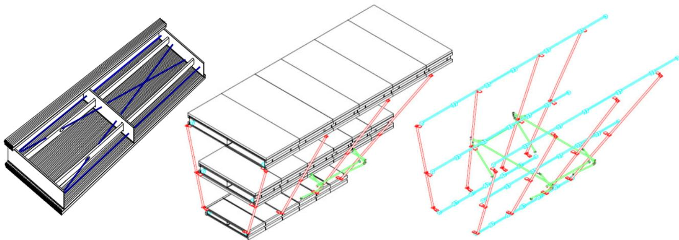
**Chamber geometry:** 20  $\mu\text{m}$  wire positioning accuracy from construction, deformations monitored by **internal optical sensors**.
