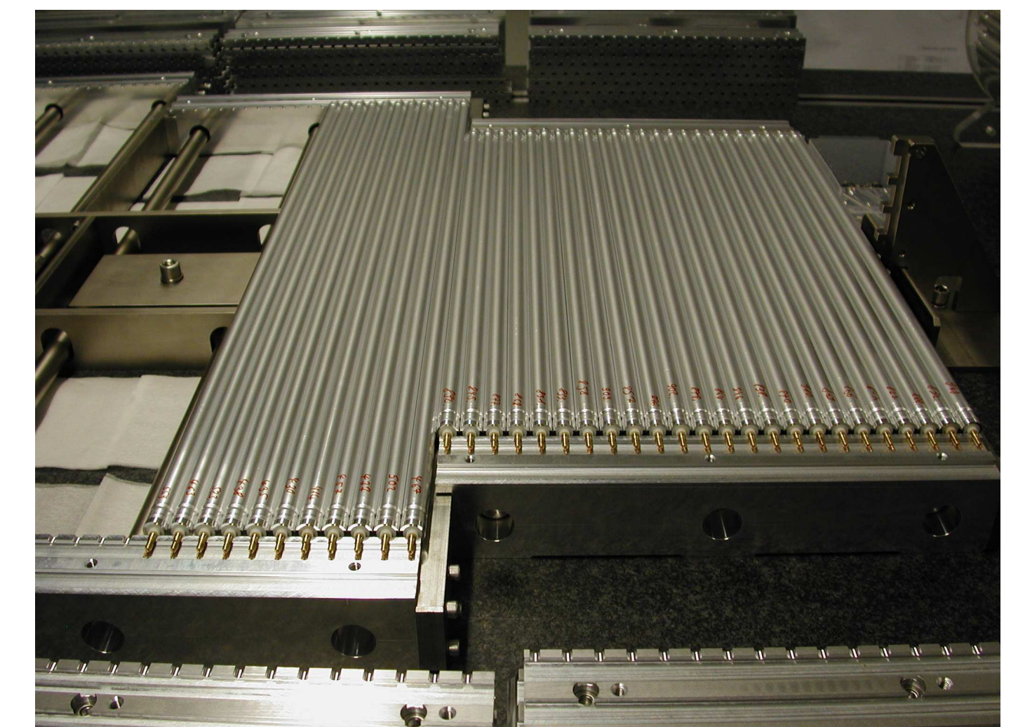
Inserting first tube layer into jigs
