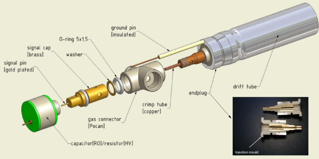
Parts (capacitor, resistor) inside insulated cans to avoid too high density of components with HV on hedgehog cards
