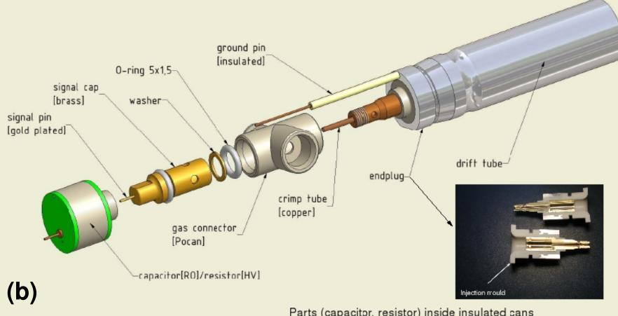
Parts (capacitor, resistor) inside insulated cans to avoid too high density of components with HV on hedgehog cards
