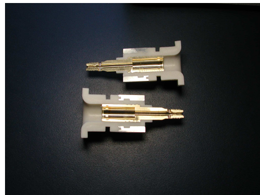
Fig. 2: Schematic drawing of the drift tube and endplug design. Photograph of a cut unmachined endplug.
