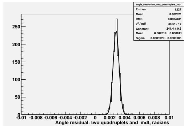
Figure 4: The distribution of the difference between the TGC and DT measured angles.
