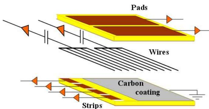
Figure 1: Schematic view of the TGC.
