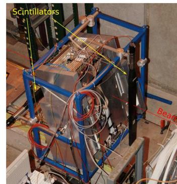
Figure 2: Prototype of a 15 mm drift tube chamber in the 180 GeV muon beam line at CERN.
