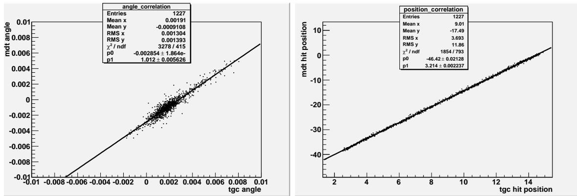
Figure 3: The correlation between the angle measured by the TGC and the angle measured by the DT (left); The correlation between the track hit position measurements (right).
