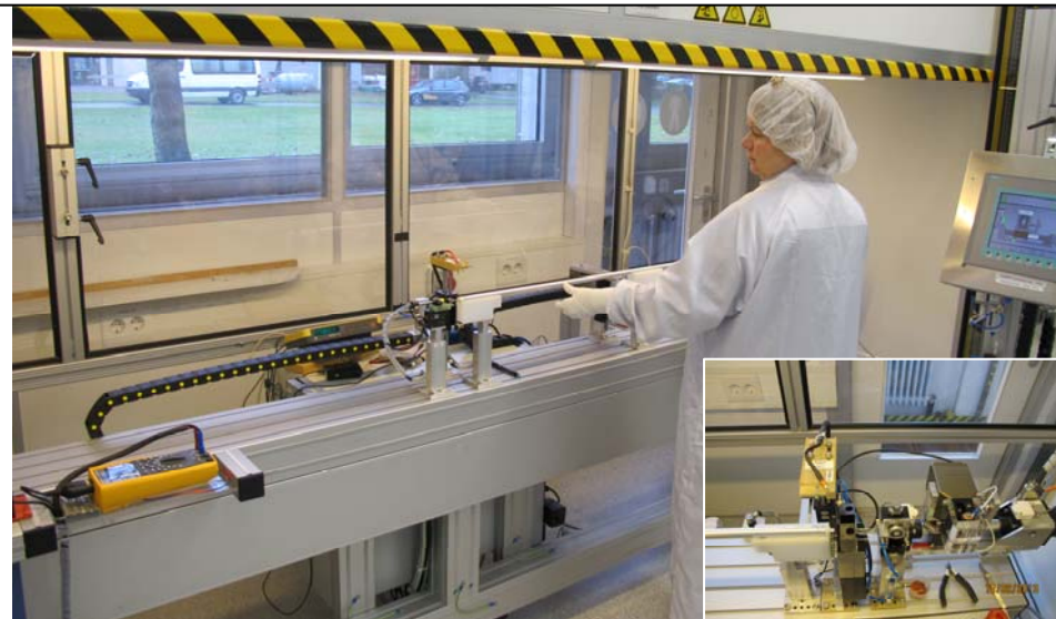
Wire tensioning and crimping + tension measurement
