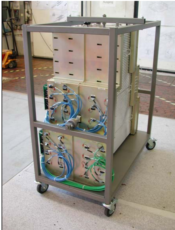
Construction of 16-layer trapezoidal prototype chamber for the inner endcap layer in 2010
