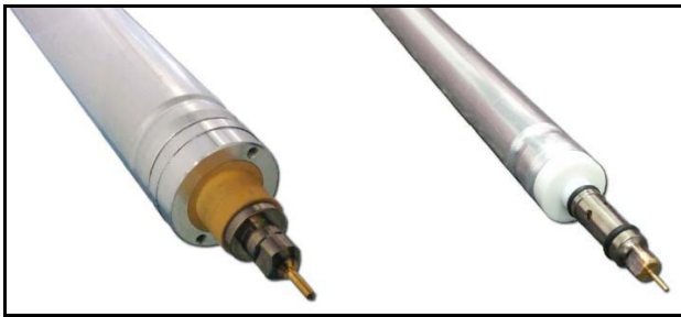
Figure 1: Comparison of the 15 mm and 30 mm diameter drift tubes of MDT and sMDT chambers, respectively (left) and of the corresponding drift time spectra with 700 ns and 185 ns maximum drift time (right).
