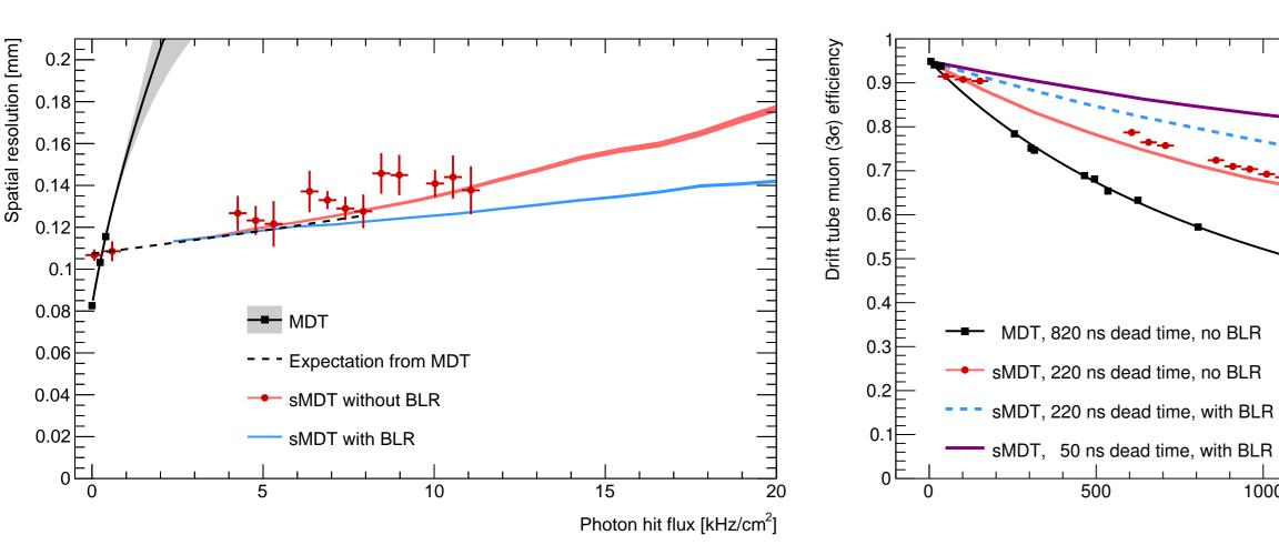
Active baseline restoration (BLR) suppresses the obsreved signal pile-up effects promising further improvement of spatial resolution and muon efficiency (hit within  $3\sigma_{resol}$  of the extapolated muon track) at high counting rates.
