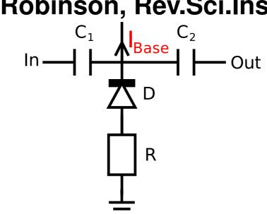
▶ Diode conducting at  $I_{Base} \neq 0$  working point.
