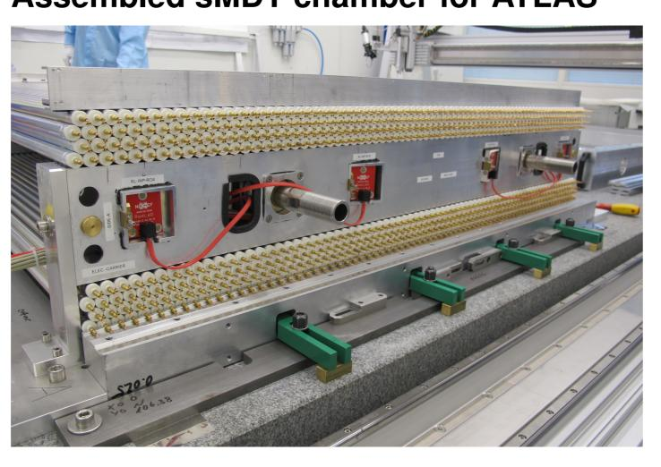
**Small-Diameter MDT chambers, sMDT:** Precision muon tracking detectors with 15 mm drift tube diameter and an order of magnitude higher rate capability than the MDTs for ATLAS upgrades and future hadron colliders.
