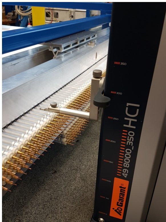
Figure 5.27: Height measurement device to measure the height of the reference surfaces of the endplugs with respect to the surface of a flat granite table.
