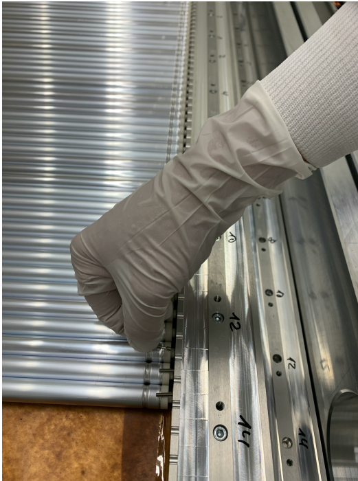
(a) Placing the grounding screws.
