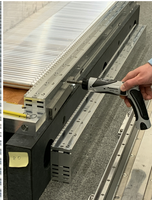
(d) Turning the grounding screws into the chamber.
