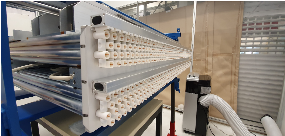
Figure 5.25: Chamber with installed gas connectors and gas distribution bars.
