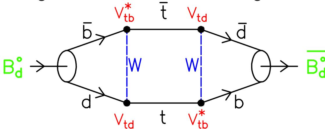
$$\Delta m_d = \frac{G_F^2}{6\pi^2} M_{B_d} m_{\text{top}}^2 F\left(\frac{m_{\text{top}}^2}{M_W^2}\right) \eta_{QCD} (f_{B_d}^2 B_{B_d}) |V_{td} V_{tb}^*|^2$$
