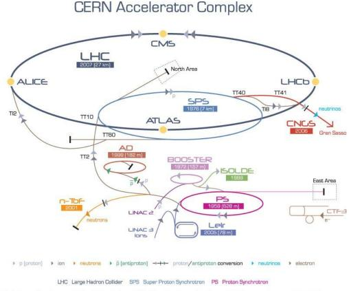
AD Antiproton Decelerator CTF3 Clic Test Facility CNGS Cern Neutrinos to Gran Sasso ISDLDE Isotope Separator OnLine Device LEIR Low Energy Ion Ring LINAC LINear ACcelerator n-ToF Neutrons Time Of Flight Instantaneous luminosity
