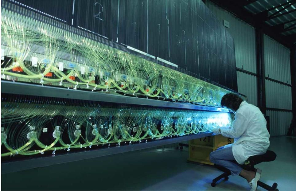
Figure 10: Part of the ATLAS hadronic calorimeter during construction.
