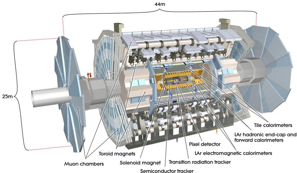
Figure 1: Cut-away view of the ATLAS detector.
