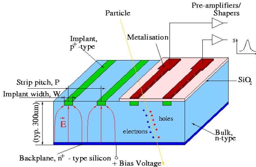
Figure 5: Schematic diagram of a *p-in-n* silicon strip detector. In a typical detector, the strip pitch would be of the order of  $\mu\text{m}$ , and the sensor thickness would be a few hundred  $\mu\text{m}$ . Individual strips can be several cm long.
