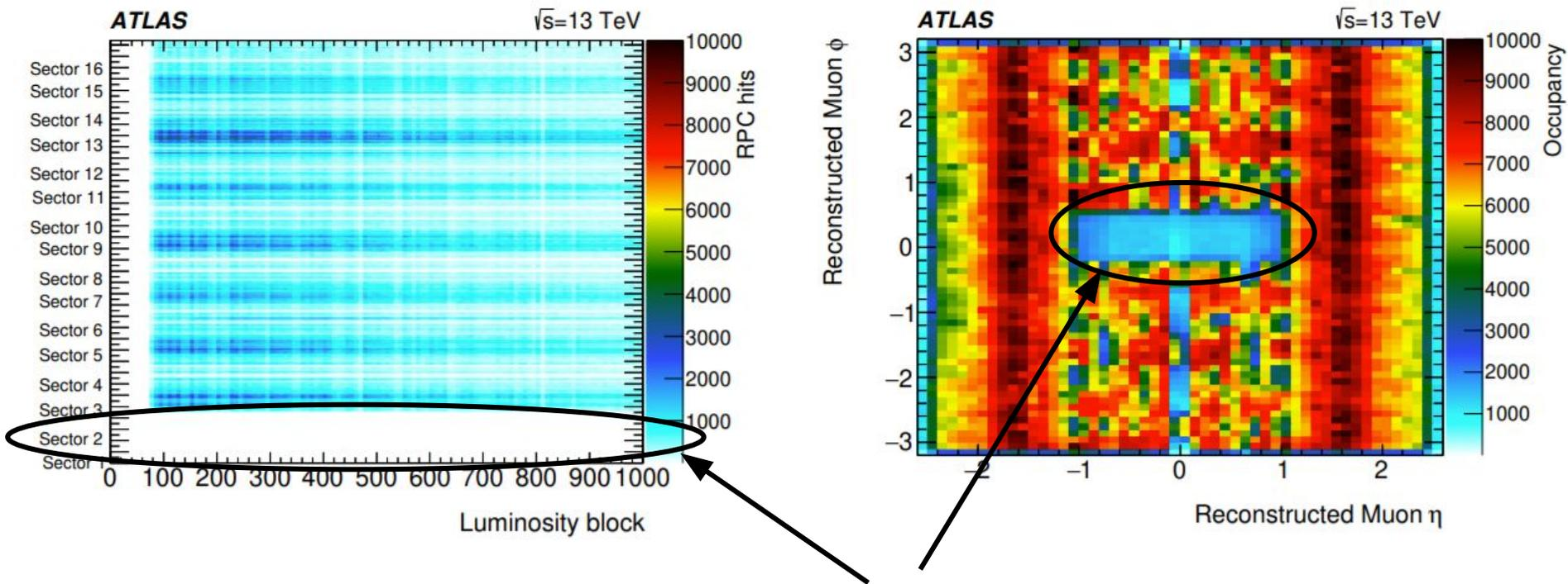
Hardware incident in muon detector during a 2017 run
