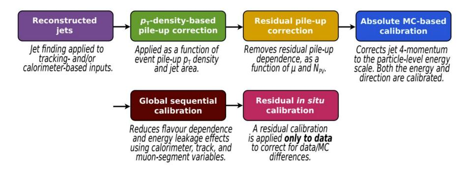
The jet energy scale calibration aims to restore the jet energy to that of jets reconstructed at the particle level
