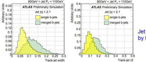
Jet substructure can be calculated by tracks or energy clusters
