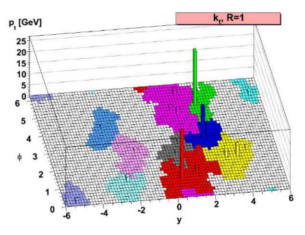
The pair with the smallest d is clustered if  $d_{ij} < d_{iB}$ , for  $d_{iB} < d_{ij}$  object i is called a jet
